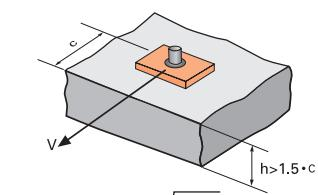
$$\Psi_{s-c,V} = \frac{c}{c_{min}} \cdot \sqrt{\frac{c}{c_{min}}}$$
