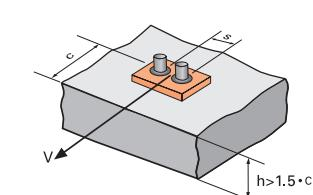
$$\Psi_{s-c,V} = \frac{3c + s}{6c_{min}} \cdot \sqrt{\frac{c}{c_{min}}}$$
