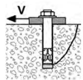
Concrete pry-out failure
